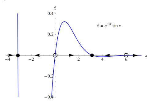
When the function is negative the flow is to the left, and when the function is positive the flow is to the right. Therefore,  $x^* = 2n\pi$  are locally unstable, and  $x^* = (2n-1)\pi$  are locally stable.
